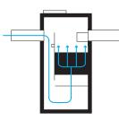
Flow Modifiers maximize sediment capture and retention by equalizing flow throughout the enhanced settling pack; its tubes provide a large surface area, small setting distances, and a controlled pollutant pathway
