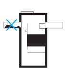
Design prevents sediment deposit in the inlet pipe
