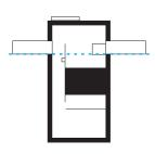
Inlet and outlet inverts can be at the same elevations
