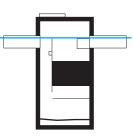
NJDEP certification assures minimal scour during peak flow events, up to 200% of the unit's treatment flow; this qualifies the unit for online use
